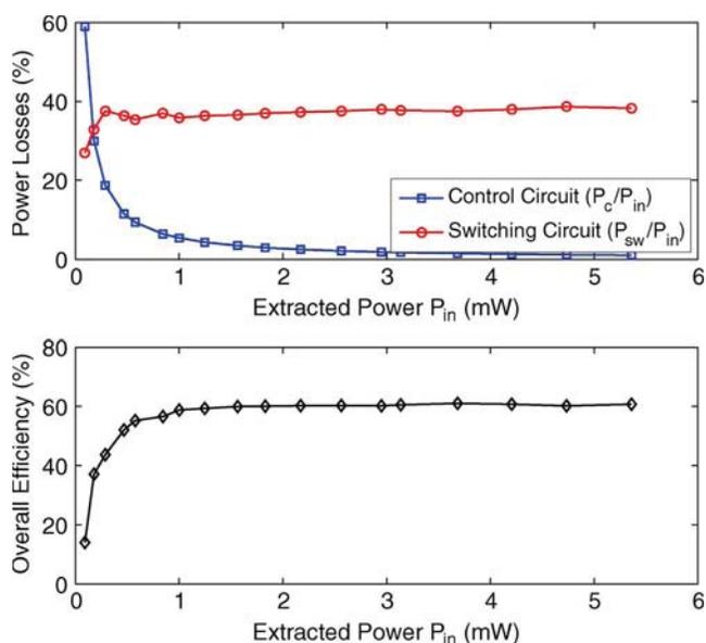
Fig. 12. Power losses and efficiency of the proposed circuit.
