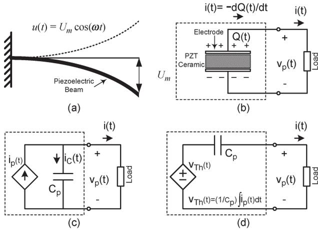
Fig. 1. (a) Schematic diagram of a vibrating piezoelectric beam (cantilever). (b) Electrical connection of the beam to a load. (c) Norton (current source) equivalent circuit of the piezoelectric energy harvester. (d) Thevenin (voltage source) equivalent circuit of the piezoelectric energy harvester.
