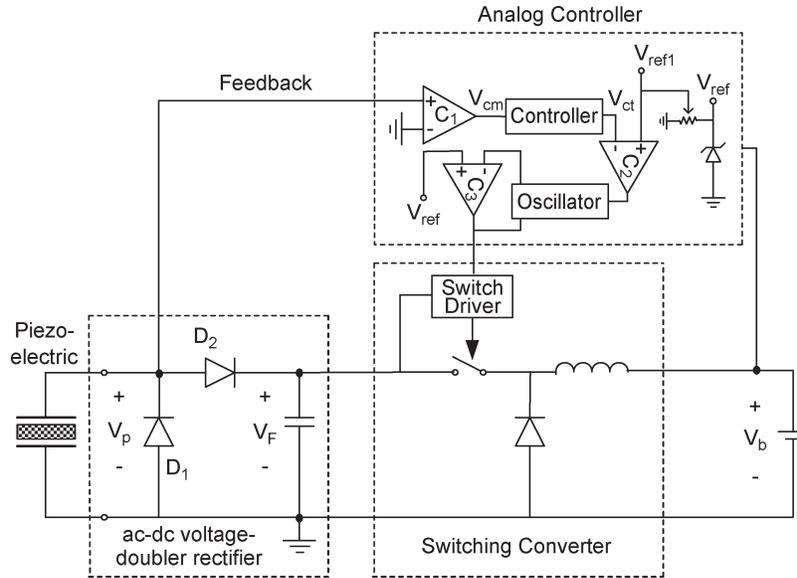
Fig. 5. Functional diagram of the proposed circuit.
