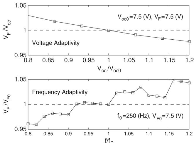
Fig. 13. Adaptivity of the controller versus voltage and frequency.
