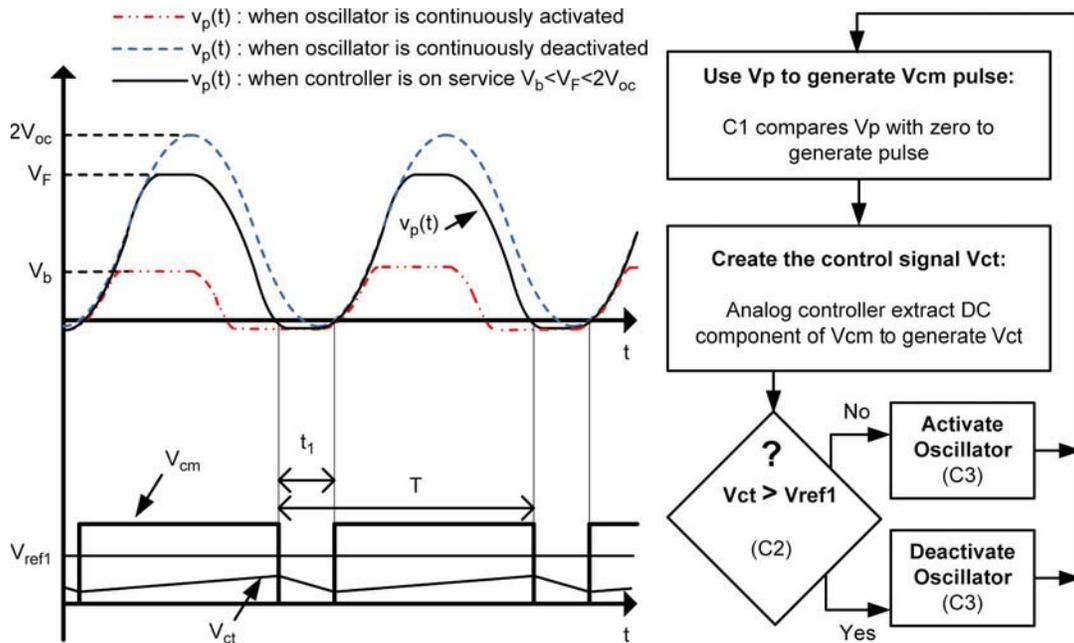
Fig. 6. (Left) Signal waveforms of the analog controller circuit and (right) the flowchart of the controller's algorithm.
