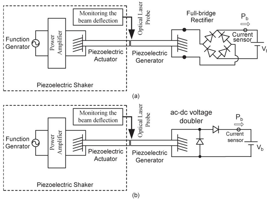
Fig. 7. Schematic diagrams of the first setup for the (a) FB and (b) VD rectifiers.
