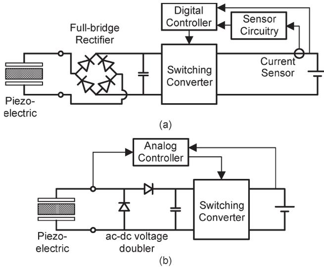
Fig. 4. Schematic diagrams for adaptive energy harvester circuits. (a) FB-based circuit using output current as a feedback. (b) Proposed circuit using piezoelectric voltage as a feedback.
