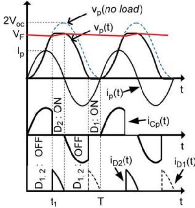
Fig. 3. Voltage and current waveforms of the VD rectifier.
