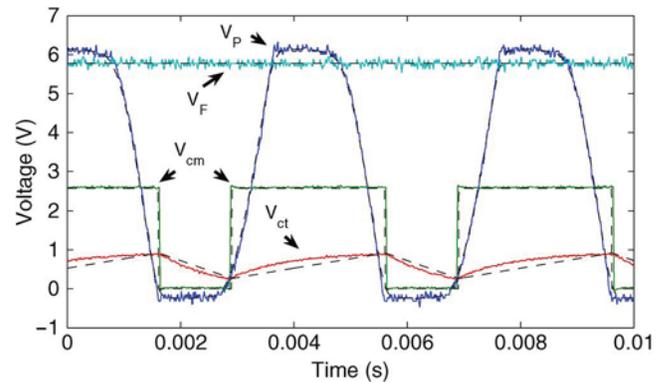
Fig. 10. (Solid lines) Captured waveforms from the experimental setup versus (dashed lines) estimated signals for analysis.
