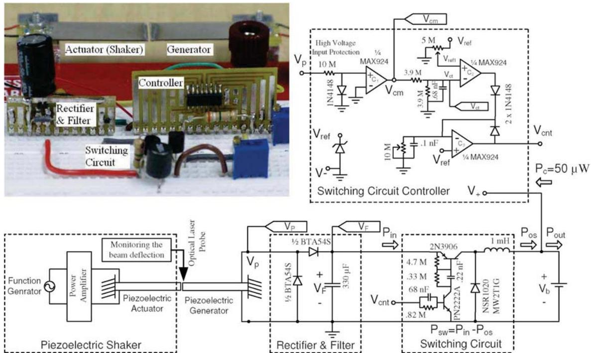
Fig. 9. Schematic diagram of the proposed low-power energy-harvesting circuit and a picture of the prototype.
