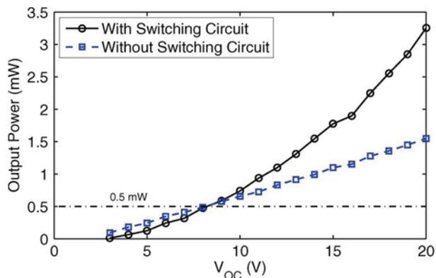
Fig. 11. Test results that compare the useful output power ( $P_{out}$ ) of the piezoelectric generator with and without the switching circuit.
